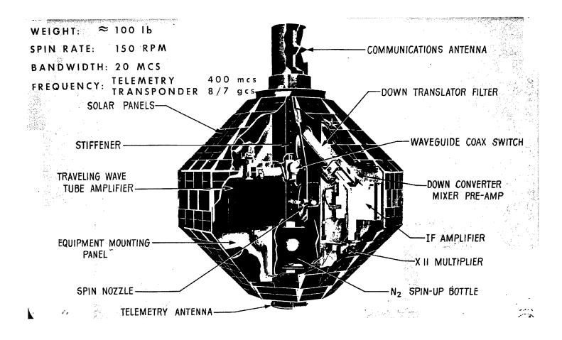
Figure 1. SPACE SUBSYSTEM - SATELLITE
