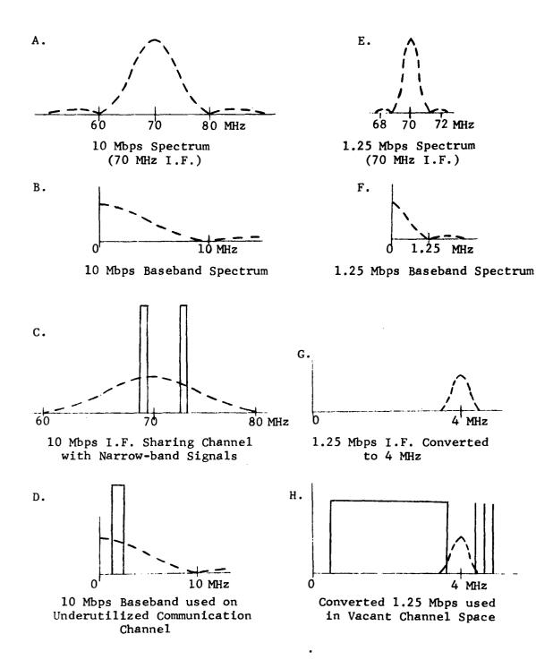
Figure 7. MODEM SPECTRA
