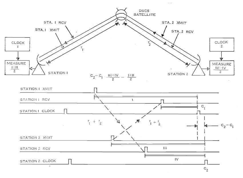
the sum of the measurements taken at the other station, the result is twice the difference between the two clocks. This method uses identical equipment and procedures at the two stations.
