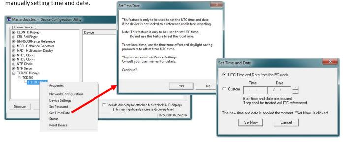
The [**Custom**] function may be most useful for demonstration, in lab situations, environments where an external signal is not available. The time for the TCD200 can either be set to the time of the PC or a manual custom time can be entered.
