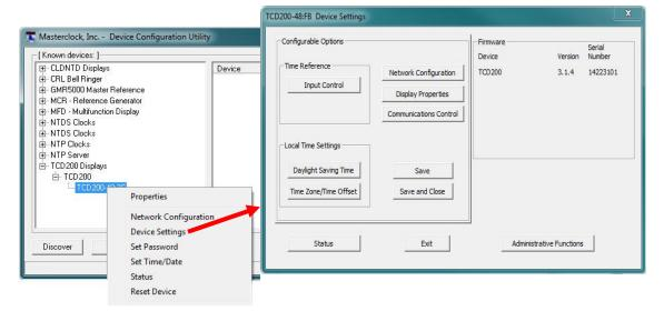
The rest of the "**Device Settings**" window includes access to all configuration options for the network. These include time reference input control, network configuration, display properties, communication control, local time settings and administrative functions, such as password. There is also a status display to monitor remote devices from your computer screen using the WinDiscovery software application.
