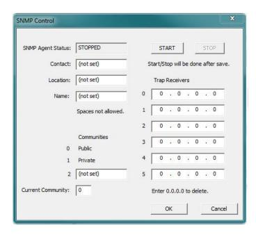
Traps are sent to the IP addresses listed as Receivers, 6 of which can be stored in the device. Not every Manager can receive traps, as such the case when an SNMP Manager is part of a multi-function utility.
