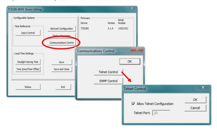
The [Communications Control] button and window enable SNMP settings.
