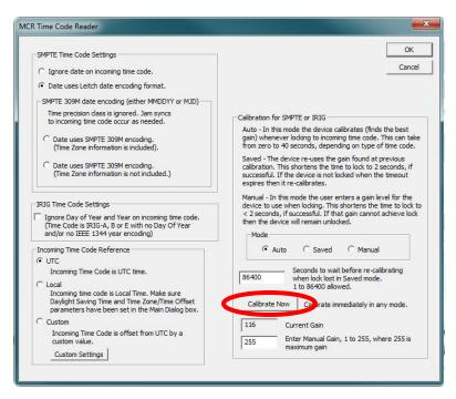
**Auto** - In this mode, the device calibrates (finds the best gain) whenever locking to incoming time code. This can take from zero to 40 seconds, depending on type of time code.
