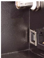
USB B port on display (back panel view)
