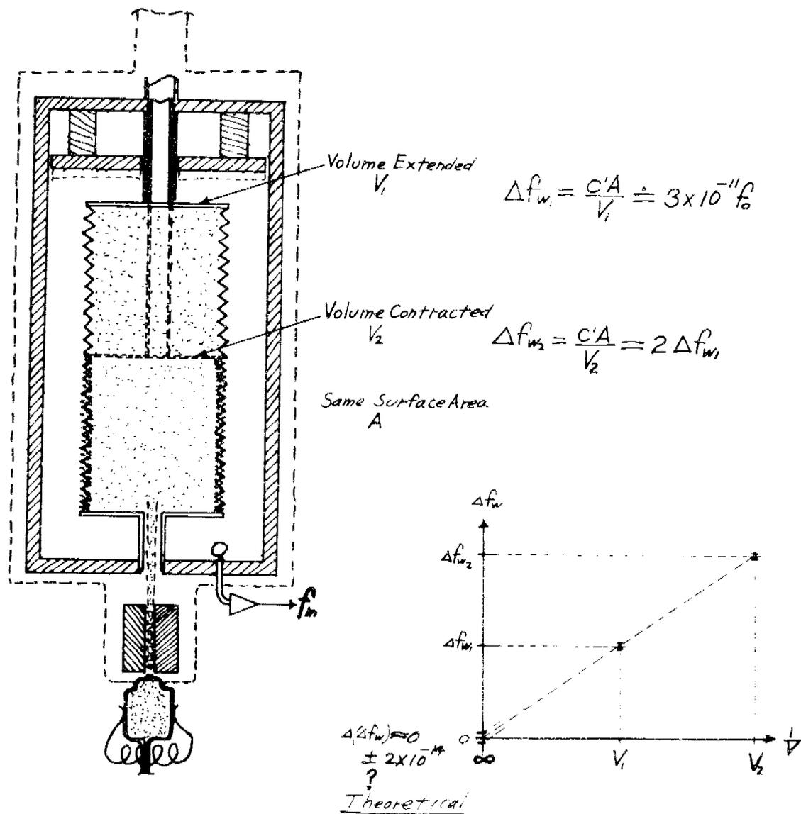
Figure 4. Variable Storage Bulb Volume Hydrogen Maser
