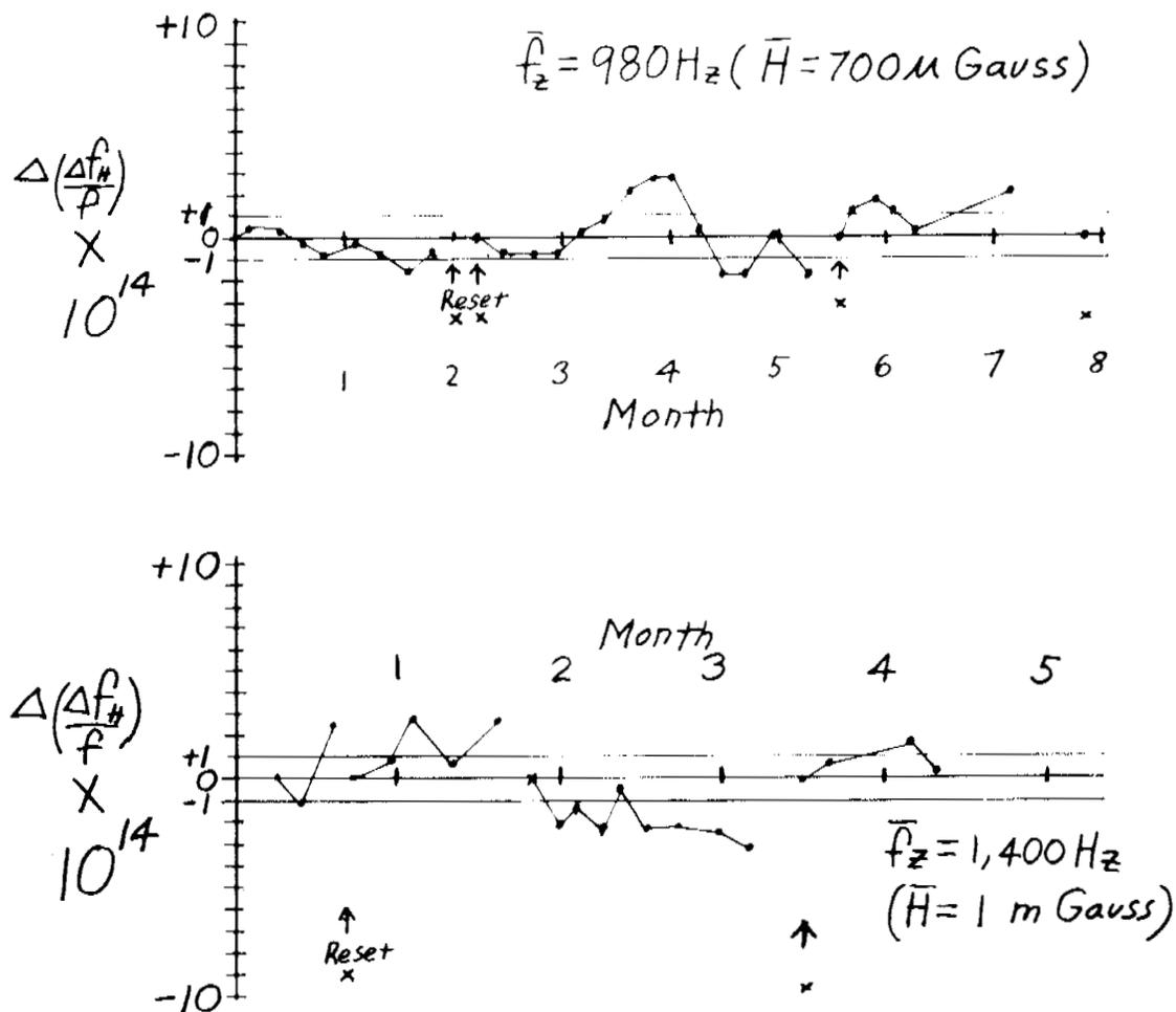
Figure 6. Magnetic Field Correction Variation NP-4 Hydrogen Maser
