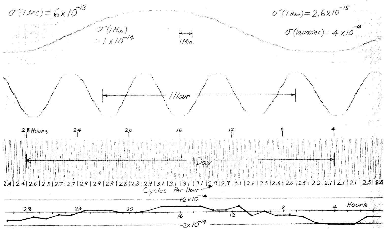
Figure 8. 9.18 GHz Phase Comparison between NP-3 and NX-2 Hydrogen Masers
