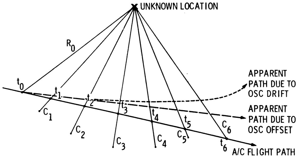
Figure 9. RANGE CHANGE PRINCIPLE AND OSCILLATOR EFFECTS
