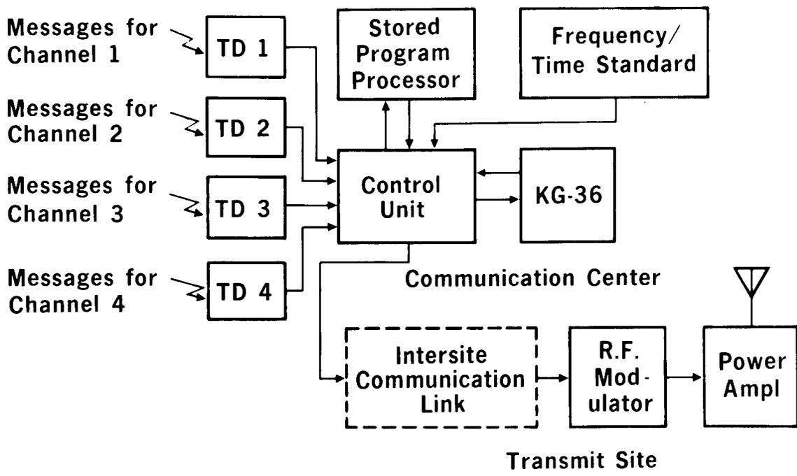
Figure 1. TRANSMIT SUBSYSTEM
