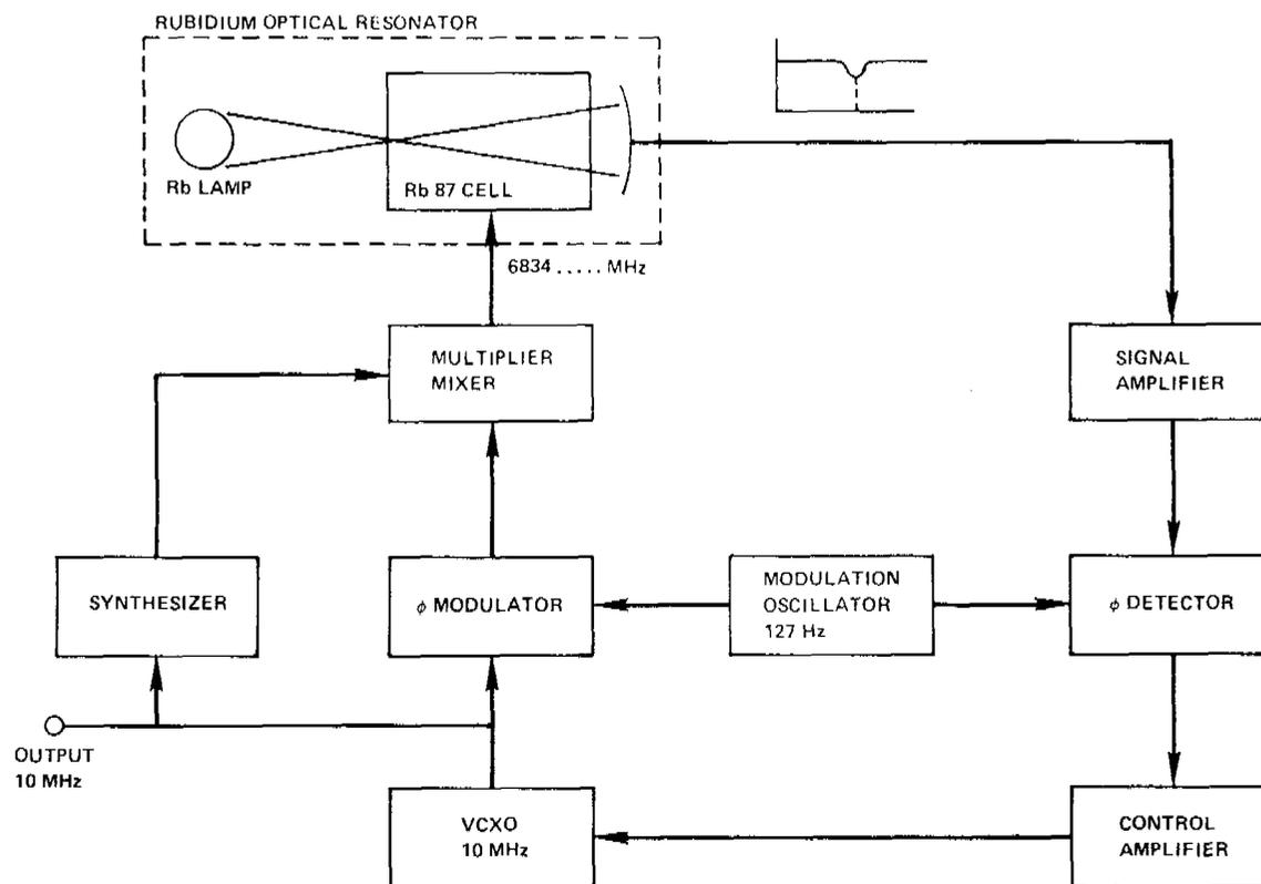
Figure 4. Block diagram of the FRK rubidium oscillator.
