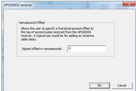
With the GPS option the GMR derives precision UTC time from satellites. The GMR includes an internal receiver that requires a pre-amplified GPS antenna.
