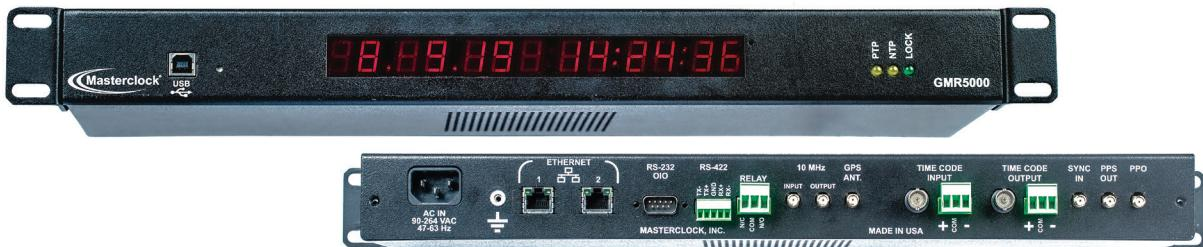
The **GMR5000** is a 1U rack mount time and frequency generator/server that can reference a variety of timing sources and provide a range of outputs to meet customer needs. The base model includes both NTP client and server functionality compatible with IPv4/IPv6 networks and offering Secure-Socket-Host (SSH) encryption for secure communications. Properly configured and using standard NTP polling rates, the device can support and synchronize thousands of simultaneous NTP clients.
