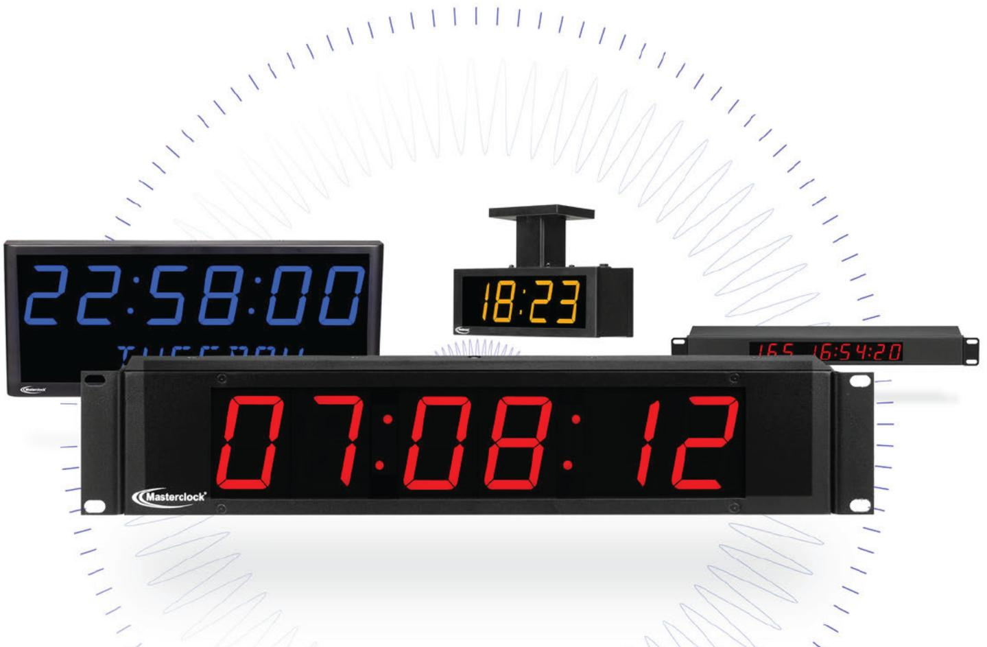
**Masterclock NTDS Digital Display** clocks sync to NTP (Network Time Protocol) or SNTP (Simple Network Time Protocol) for accurate and traceable time. Power over Ethernet (PoE) included. Configure to time zone and Daylight Saving Time parameters.
