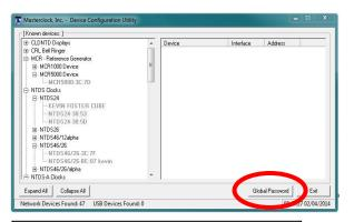
The **Global Password** being used must match the password on all the devices being administered. On any new system being installed, the factory default password on all devices is "public".
