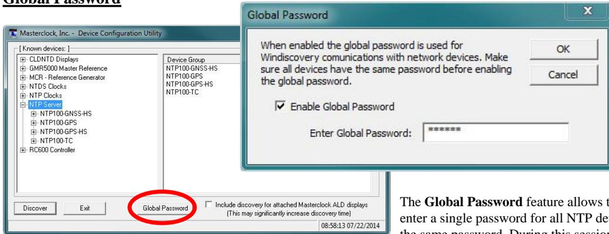
The **Global Password** being used must match the password on all the devices being administered. On any new system being installed, the factory default password on all devices is “**public**”.
